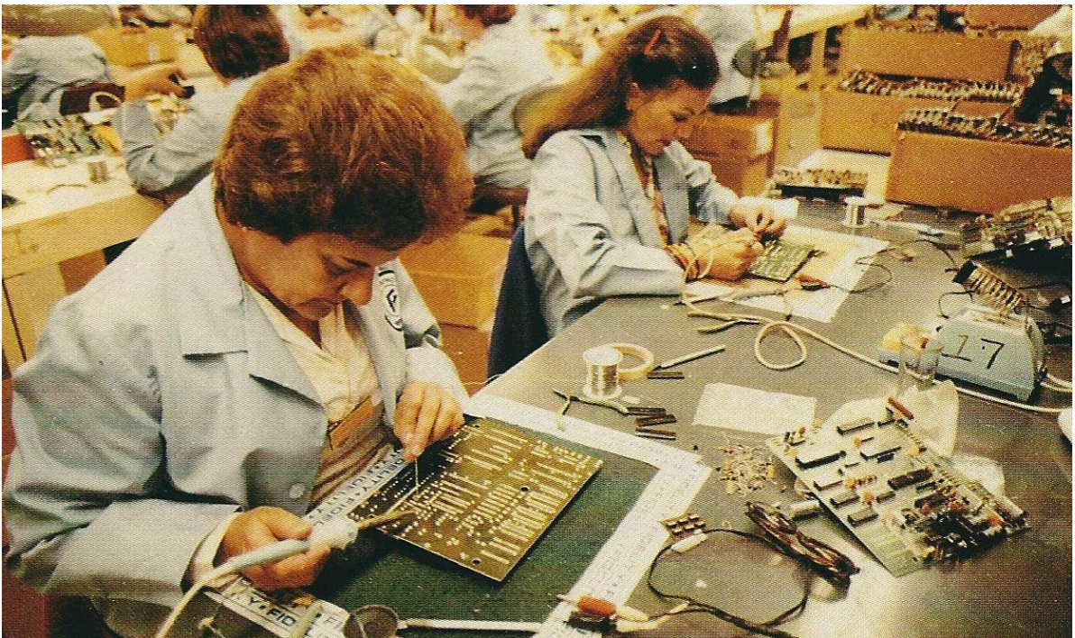
During the early Chess Challenger era, Fidelity's production capacity reached up to 250 printed circuit boards per day, reflecting one of the more efficient phases of their manufacturing process.
