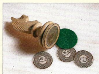
■ Electronics for piece recognition
