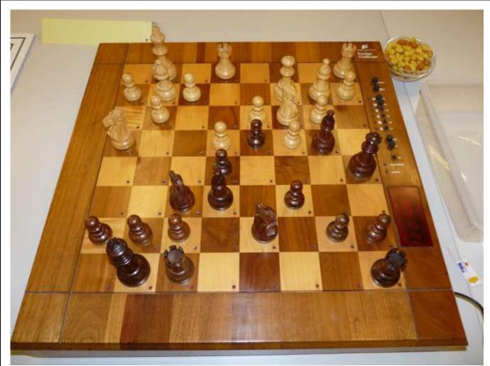
An early model of the **Fidelity Prestige with the flat display** at the 30th CSVN (simultaneous) users tournament in Leiden (13 June 2015). This Prestige was upgraded with the Avant Garde 2 program running on a 68000 Motorola 16MHz processor. First owner the Dutch chess computer expert Jan Louwman, second owner Rob van Son. The Prestige won 'the best move trophy.' The simultaneous display against 12 chess computers was given by Prof. Dr. Jaap van den Herik and IM Hans Böhm.
