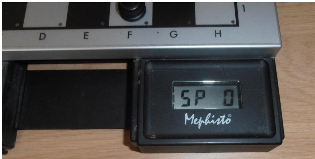
SP = Spare Time. This restores time control in the event of a power failure or crash.
